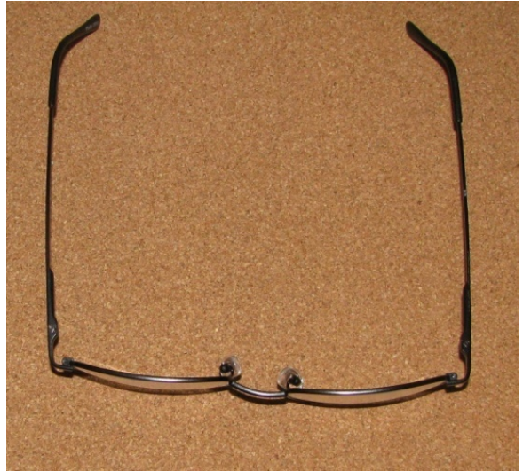
Skewed out of coplanar alignment
